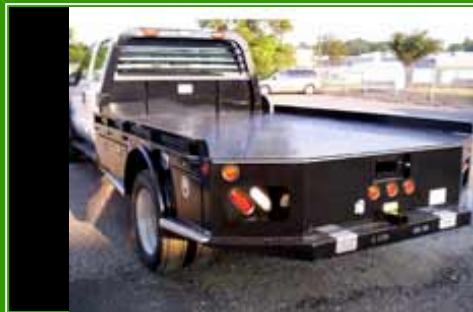
F450 CC 4x4 , Blue Ridge Super Hauler 9.5' DRW; 96" Width. Trailer Plugs(2), Receiver Hitch, Goose neck hitch compartment w/ball.
